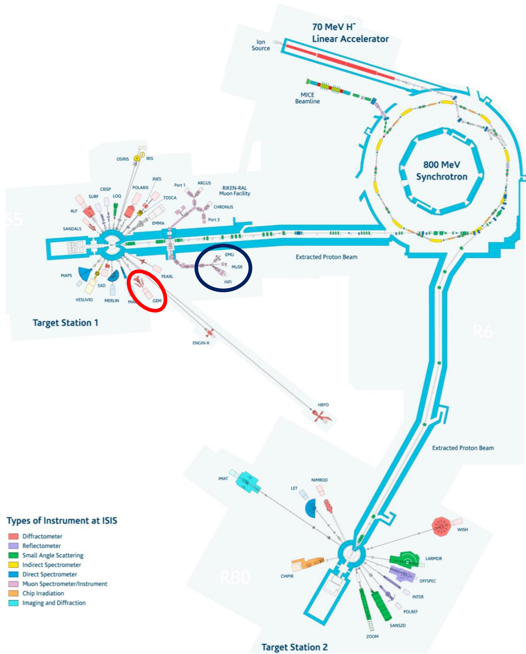
Figure 3.8: Schematic layout of the ISIS spallation neutron and muon source showing the approximate locations of all the end stations. The GEM diffractometer is highlighted by a red circle and the \mu SR end stations are highlighted by a blue circle. Taken from [13].
