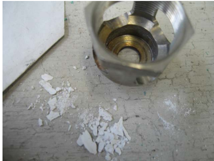
Figure 3.6.6e Manual cleaning of injector sleeve with tweezers.
