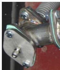
Figure 3.2.7 Capped T-joint with pressure tapping.
