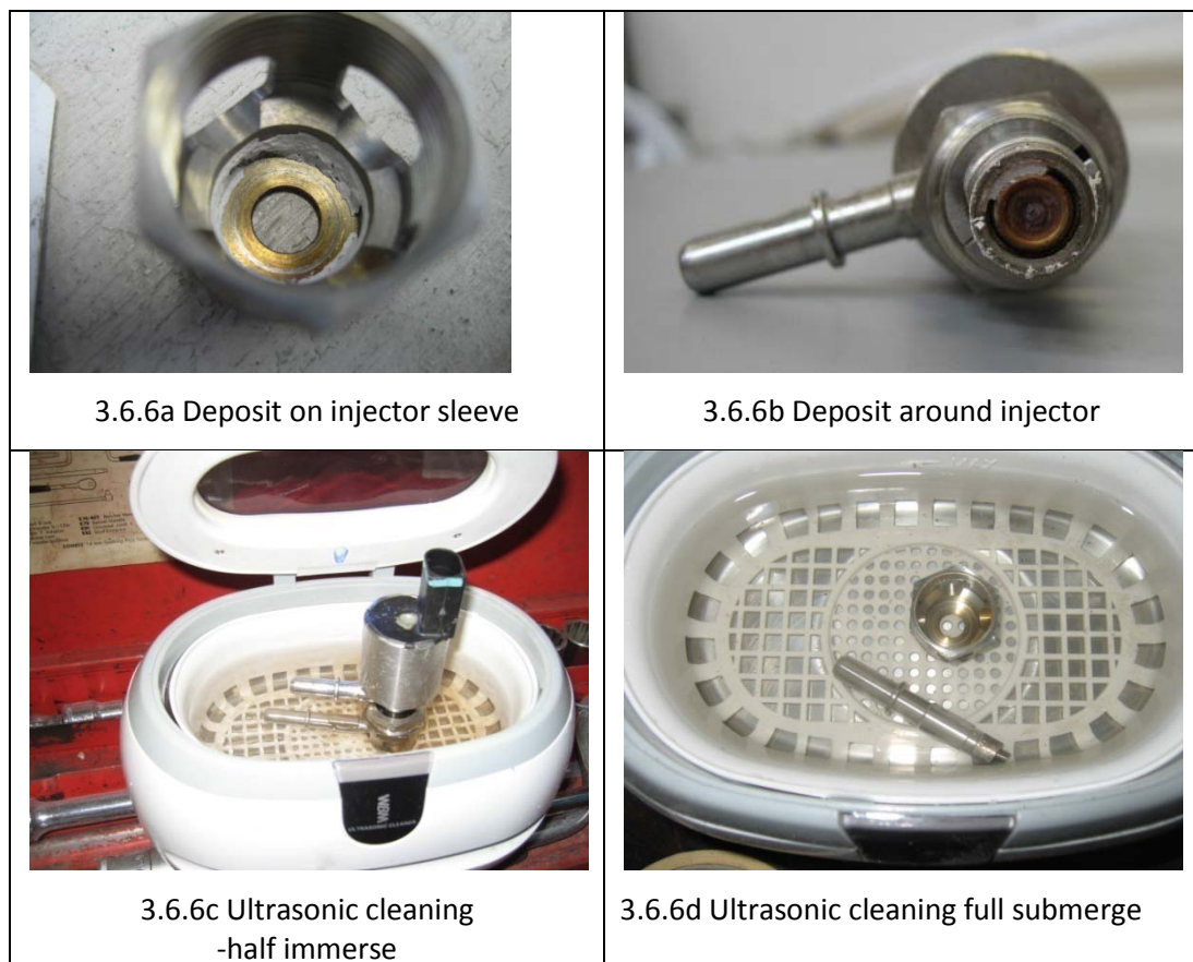
Figure 3.6.6 White deposit build up and ultrasonic cleaning
