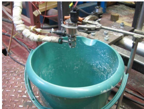
Figure 3.6.4a Urea AdBlue Injector testing prior to experimental with spray system.
