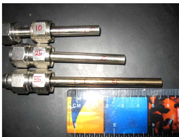
Figure 3.9a Variation of sampling probe length for profile measurement
