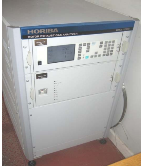
Figure 3.4 The MEXA-1170Nx NH 3 Analyser Unit
