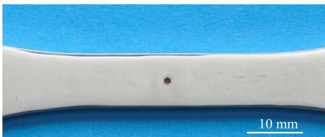
FIGURE 4 Close-up view of a pre-pitted specimen. The pit width (diameter) is 520\ \mu\text{m} and pit depth is 174\ \mu\text{m} [Colour figure can be viewed at wileyonlinelibrary.com ]
