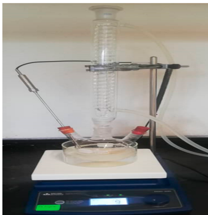
Figure 2. Batch reactor experimental setup.
