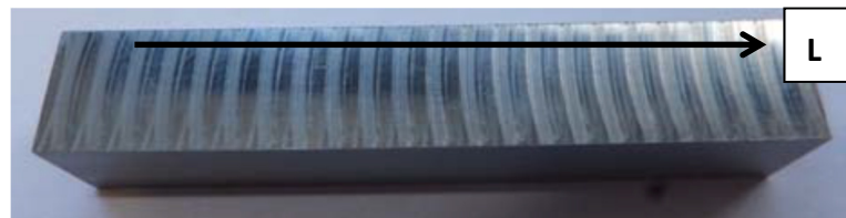
Figure 2. Sample 24. Manufacturing grooves can be clearly seen. Longitudinal orientation is indicated.
