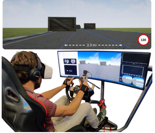
Fig. 4. Driving simulator setup. Top: simulated environment with an overlay of the three virtual lanes considered, their width and the free-flow speed. Note that none of these overlays were visible to participants during the experiment. Bottom: the participant wears a VR headset with integrated eye tracker. The screen shows the scene displayed to the participant and real-time sensor readings for monitoring purposes.
