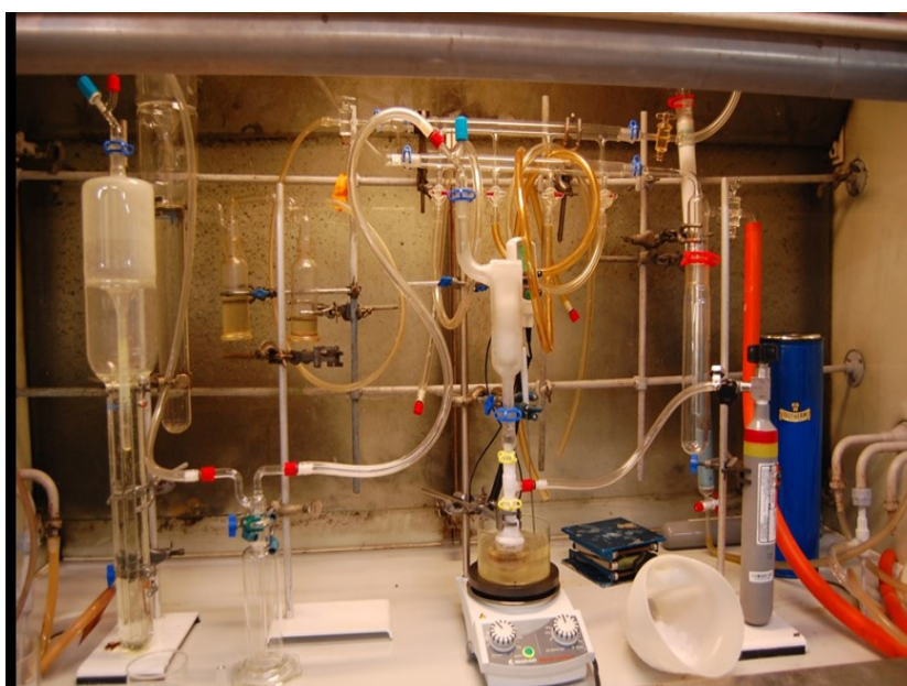
Figure 2.33: Small-scale experimental apparatus; bio-derived thiophene synthesis.
