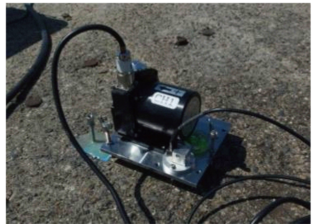
FIGURE 3 | Installation of velocity meter.
