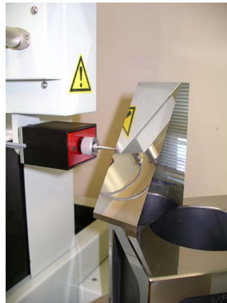
(a) Measurement of plane S_4 using dial gauge to realize basic posture
