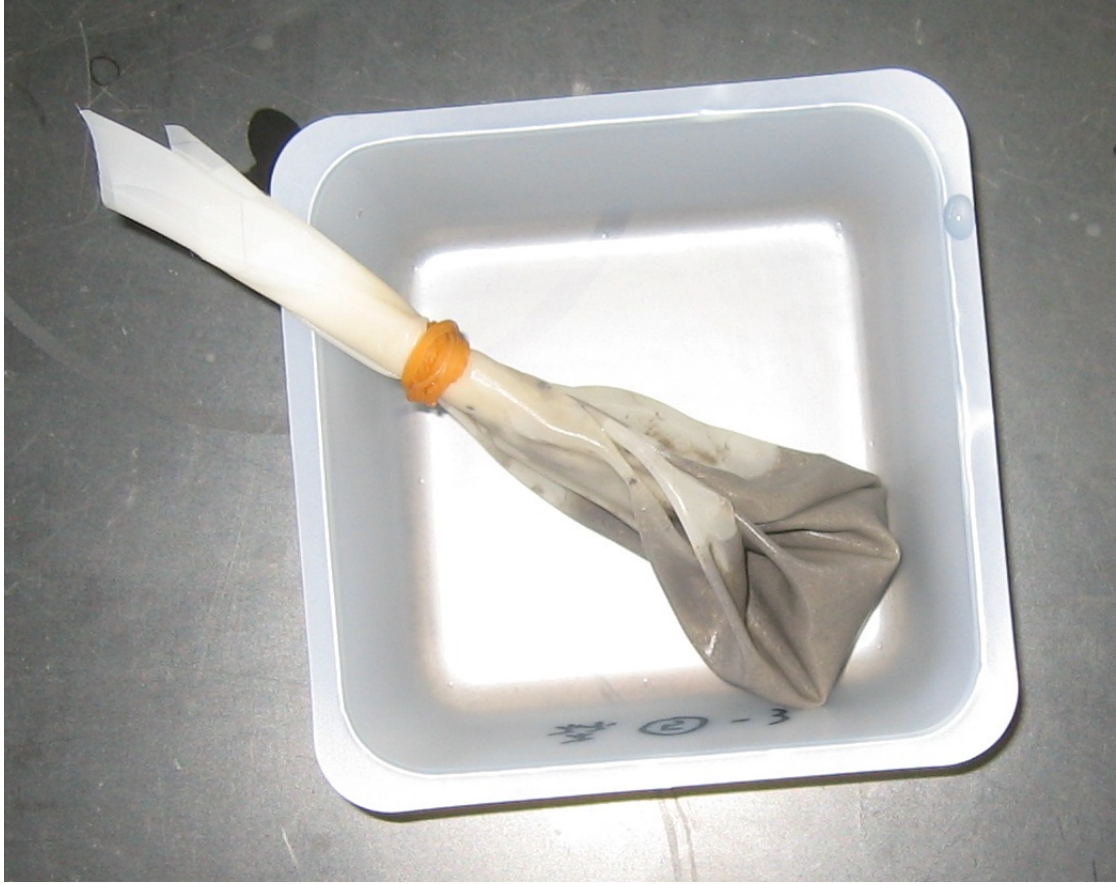
Figure 1: A picture showing a soil sample packed in the nylon mesh cloth. The sample is already washed with tap water.
