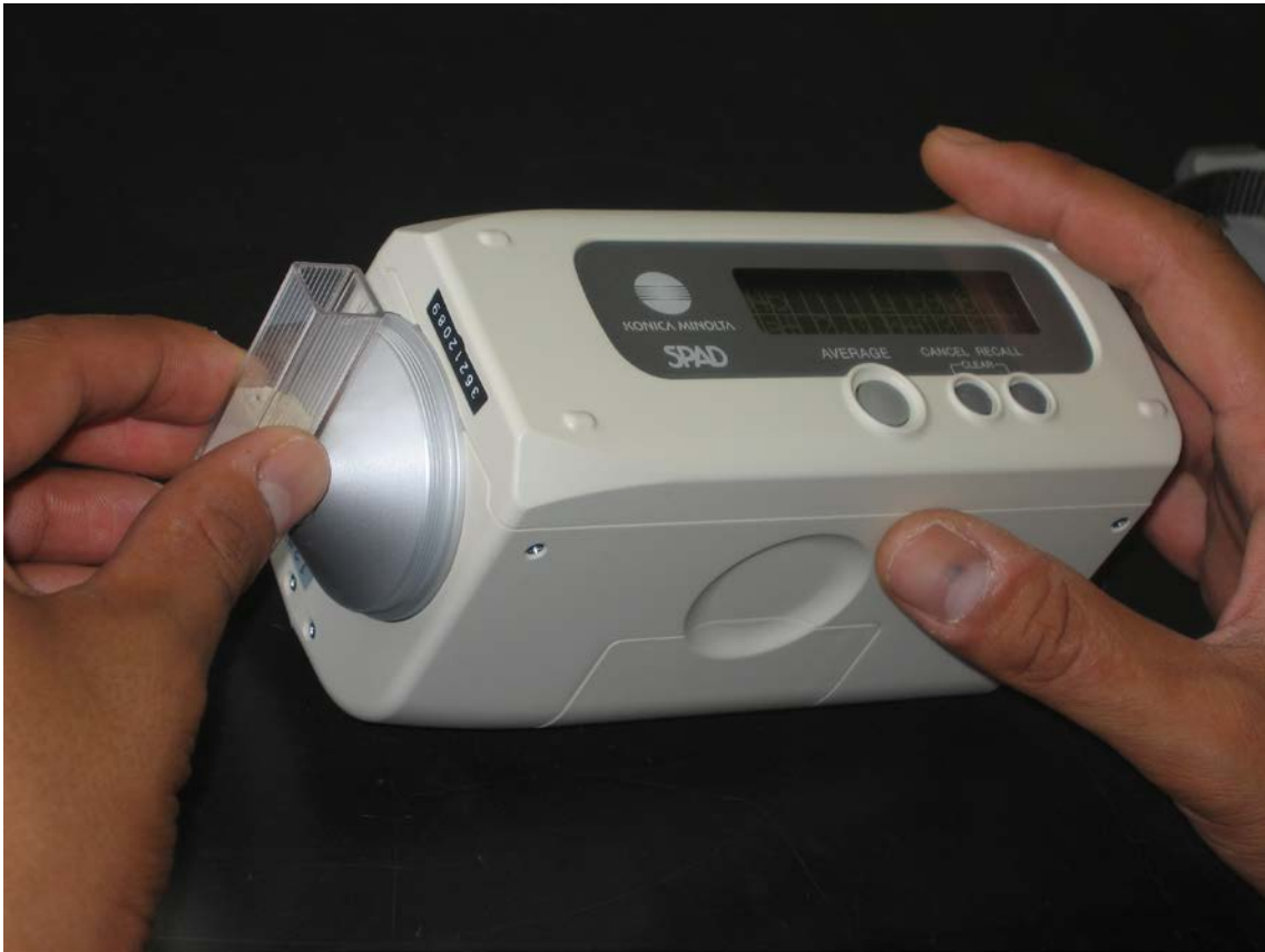
Figure 1: A picture showing measurement of a soil sample packed in a plastic cell with SPAD-503.
