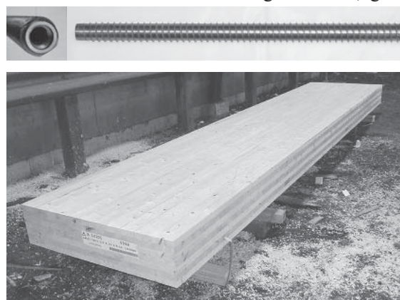
Figure 1. Shape of a Lagscrewbolt and Cross Laminated Timber
