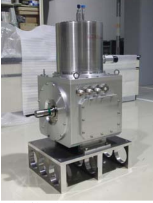
Fig. 6. Photographs of low thermal invasion cryostat for the testing 2 nd generation HTS-ISM (Fig. 4).
