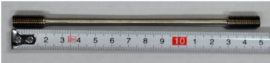
Figure 1. Photograph of an SEA bar test specimen.
