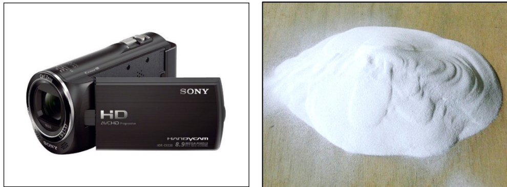
Figure 3-4. (left) The camera used for recording the continues images; (right) White PVC tracer particles
