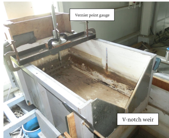
Figure 4-5. V-notch weir and Vernier point gauge for controlling water discharge
