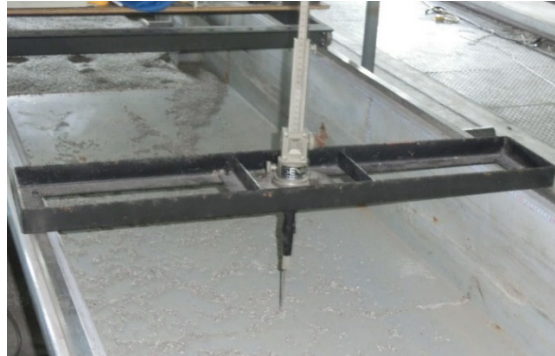
Figure 4-7. The Vernier point gauge used for measuring the water level in different cross sections along the channel.
