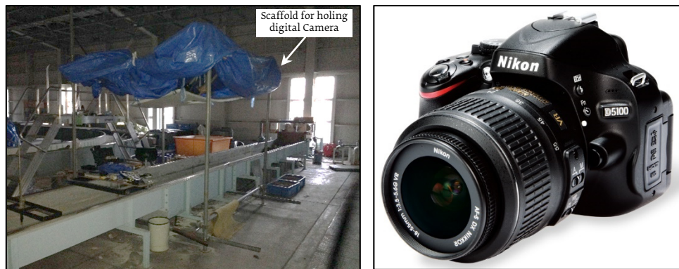
Figure 4-10. The scaffold mounted for holding the digital cameras (right photo) which were used for monitoring bed form migration
