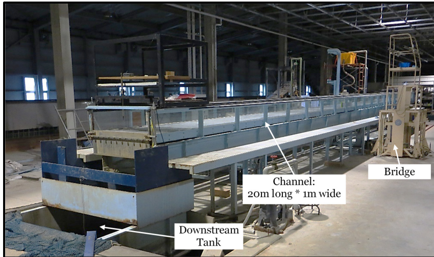
Figure 3-1. A view of channel used for fixed bed experiments
