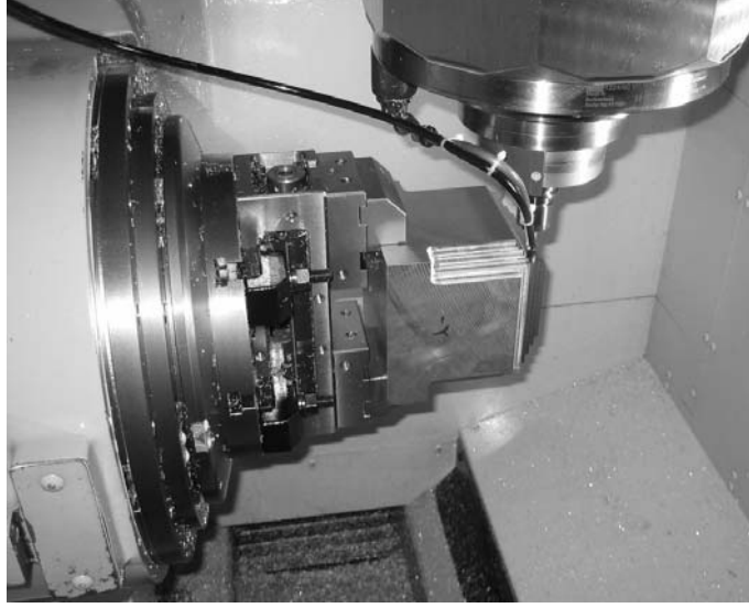
Figure 6: Machining test setup (at B = -90^\circ ).
