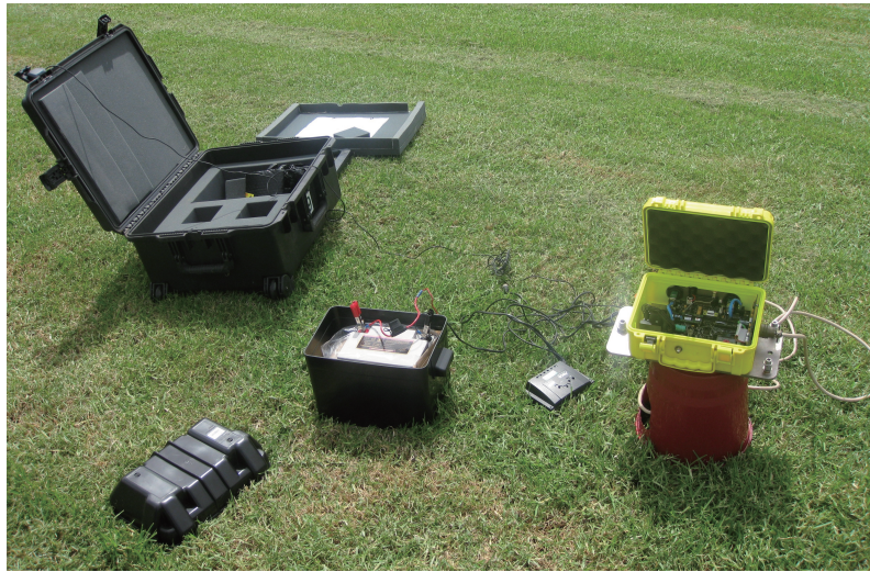
Figure 3.2: Set up on a single station. The three-component seismometer is covered with the bucket.
