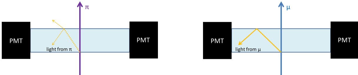
Figure 4.5: Illustration of light propagation in Cherenkov detector for pion (left) and muon (right).
