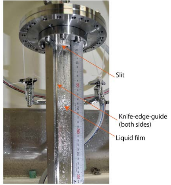
Fig. 3. Overall view of the experimental setup.
