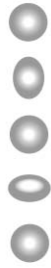
Fig. 1. Simulation model of modal deformation of a droplet, oscillating at basic mode (n=2) of natural frequency. It shows an axisymmetric deformation.
