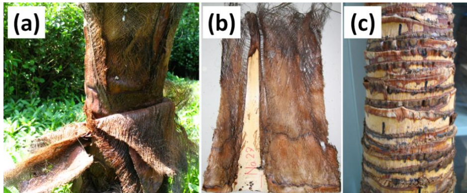
Figure 6.2 Photographs of windmill palm showing lignified fibrovascular bundles in leaf and stem: (a) windmill palm stem surrounded by many layers of leaf sheaths (at a height of 1.5 m), (b) one leaf sheath taken from a windmill palm, (c) windmill palm stem after all leaves have been pilled. (Zhai et al. 2012)
