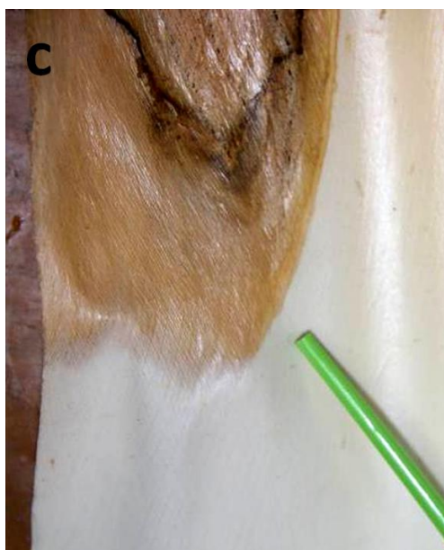
Figure 3.1 Leafs from windmill palm. a: Leaf No. 31 & 32, which show dark brown color over all sheath and detached fibers. b: Leaf No. 21 & 22, which show changing color from bottom to top part. c: Transition parts (a twig pointed area) between living and non-living tissues in leaf sheath of leaf No.18.
