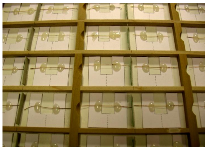
Figure 2.11 Specimens under 60% relative humidity and 20°C condition.
