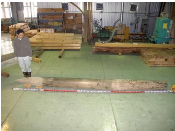
Photo 5 Wood pile retrieved from Kida Bridge
