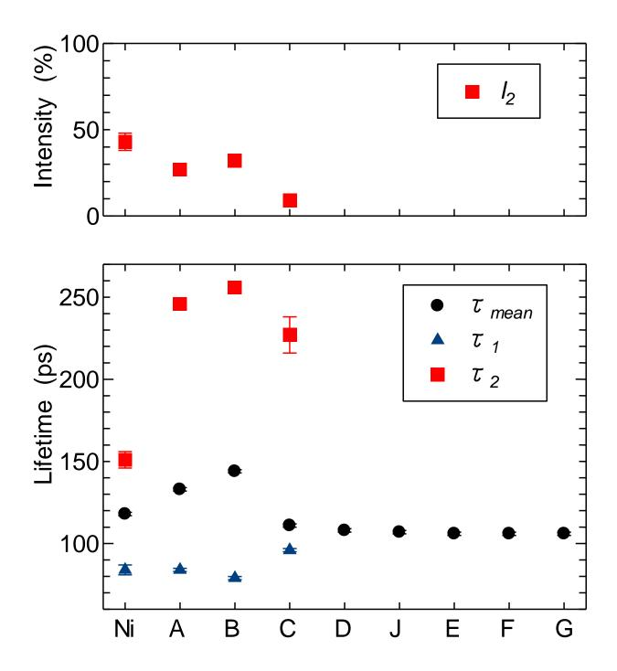
Figure 2 Positron annihilation lifetimes of electron irradiated Ni, model alloys and commercial alloys of austenitic stainless steels at 573 K to a dose of  $1.5 \times 10^{-2}$  dpa.  $\tau_{\text{mean}}$  is the mean life time, and  $\tau_1$ ,  $\tau_2$ ,  $I_2$  are the short lifetime, long lifetime and the intensities of the long lifetime, respectively.
