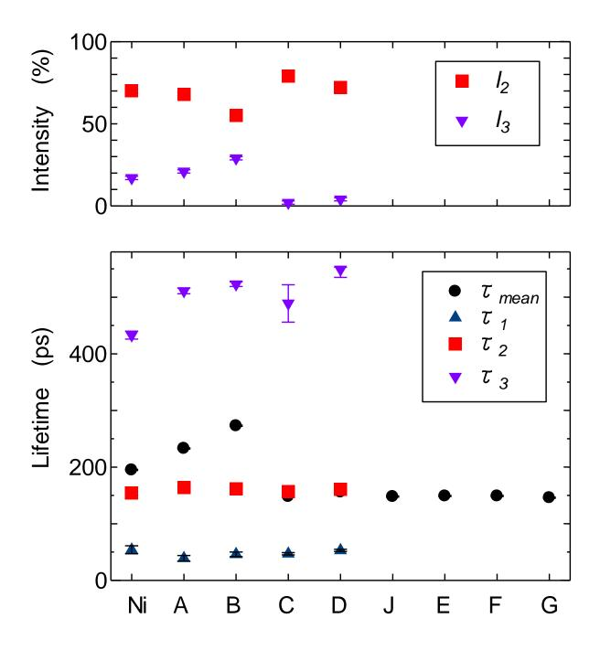
Figure 5 Positron annihilation lifetimes of neutron irradiated Ni, model alloys and commercial alloys of austenitic stainless steels at 573 K to a dose of 0.2 dpa.  $\tau_{\text{mean}}$  is the mean lifetime,  $\tau_1$ ,  $\tau_2$ ,  $\tau_3$ ,  $I_2$  and  $I_3$  are the short lifetime, two long lifetimes and the intensities of the two long lifetimes, respectively.
