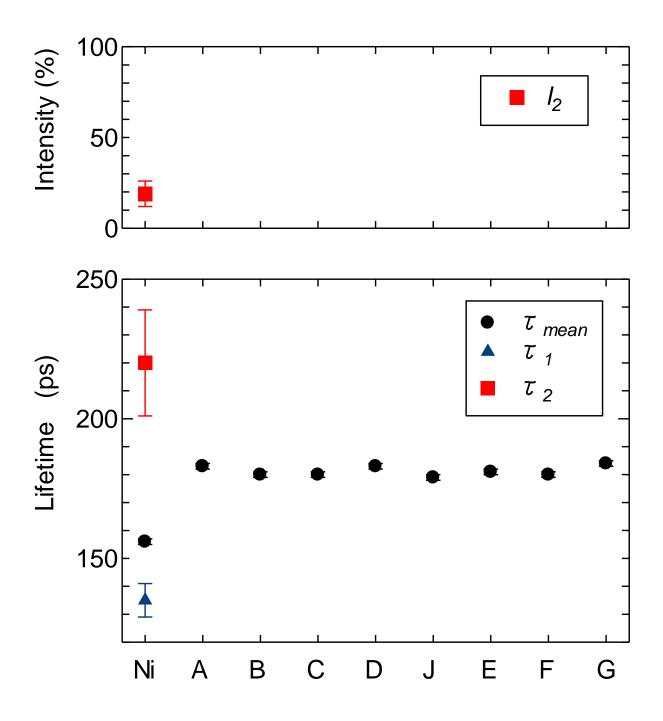
Figure 1 Positron annihilation lifetimes of electron irradiated Ni, model alloy and austenitic stainless steels at 343 K to a dose of  $1.2 \times 10^{-2}$  dpa.  $\tau_{\text{mean}}$  is the mean lifetime, and  $\tau_1$ ,  $\tau_2$  and  $I_2$  are the short lifetime, long lifetime and the intensity of the long lifetime, respectively.
