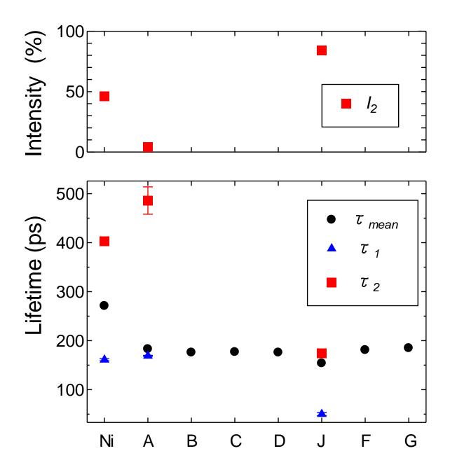
figure 3 Positron annihilation lifetimes of neutron irradiated Ni, model alloys and austenitic stainless steels at 363 K to a dose of 0.2 dpa.  $\tau_{\text{mean}}$  is the mean lifetime, and  $\tau_1$ ,  $\tau_2$  and  $I_2$  are the short lifetime, long lifetime and the intensity of the long lifetime, respectively.
