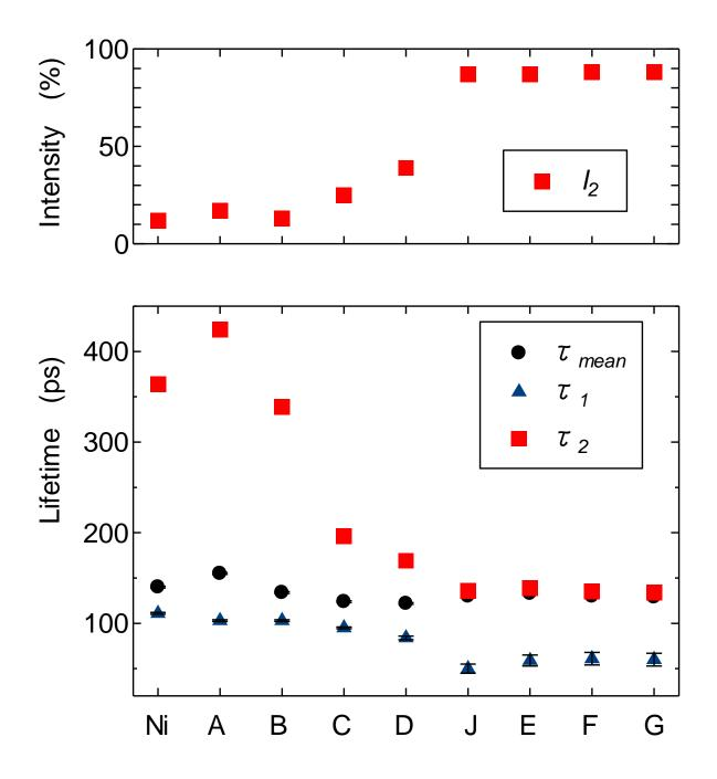
Figure 4 Positron annihilation lifetimes of neutron irradiated Ni, model alloys and austenitic stainless steels at 573 K to a dose of  $1.6 \ge 10^{-3}$  dpa.  $\tau_{\text{mean}}$  is the mean lifetime, and  $\tau_1$ ,  $\tau_2$  and  $I_2$  are the short lifetime, long lifetime and the intensity of the long lifetime, respectively.
