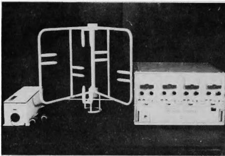
Fig. 5. The improved type of sonic anemometer-thermometer in all solid state circuit, which measures three dimensional components of wind velocity and air temperature. The three sound paths are 20 cm in length and two horizontal ones are crossing in 120°.
