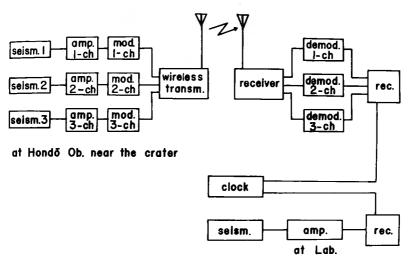
Fig. 2. Block diagram of telemetering system.
