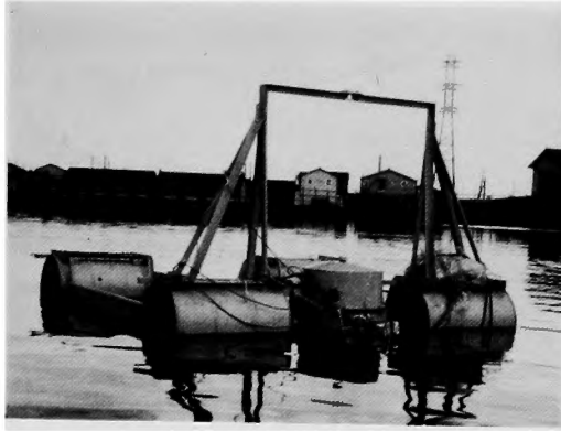
Fig. 6. The new evaporimeter on the reservoir.
