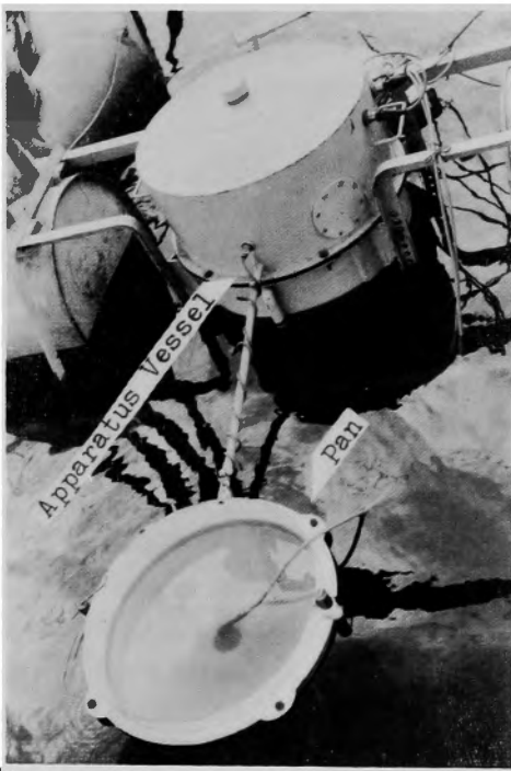
Fig. 3 The pan and the apparatus vessel on the side of the raft.
