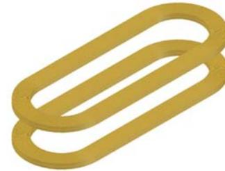
Fig. 8. Dipole magnet consisting of a pair of stacked two racetrack coils.
