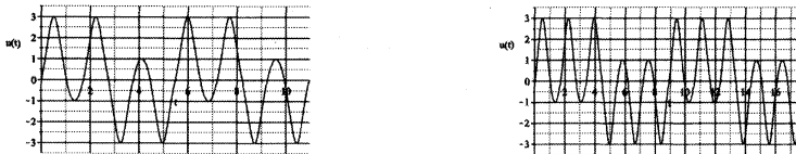
Figure 4.5: (left):The time history of the “triple-time oscillations” orbit with the initial condition: u(0) = 0, \dot{u}(0) = \sqrt{30} . The time is shown up to two periods. \omega \doteq 5.4755 . (right): The time history of the “quintic-time oscillations” orbit with the initial condition: u(0) = 0, \dot{u}(0) = \sqrt{30} . The time is also shown up to two periods. \omega \doteq 8.9036 . The orbits of both figures are the same of Figure 4.2 and/or 4.3.
