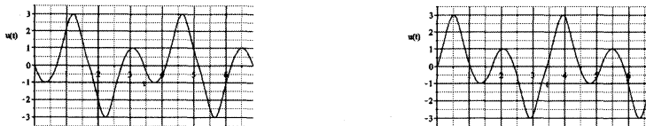
Figure 4.6: (left):The time history of the “double-time oscillations” orbit with the initial condition: u(0) = 0, \dot{u}(0) = -\sqrt{30} . The time is shown up to two periods. \omega \doteq 3.428 . (right): The time history of the “double-time oscillations” orbit with the initial condition: u(0) = 0, \dot{u}(0) = \sqrt{30} . The time is also shown up to two periods. The orbits of both figures are the same of Figure 4.2 and/or 4.3.
