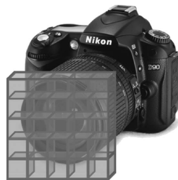
Fig. 7 Due to variable angle of incidence of light, band-pass filter behaves as dozens of small band-pass filters connected to each other
