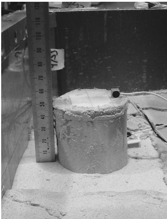
Fig. 8. Uplifted manhole after shaking (CS3)
