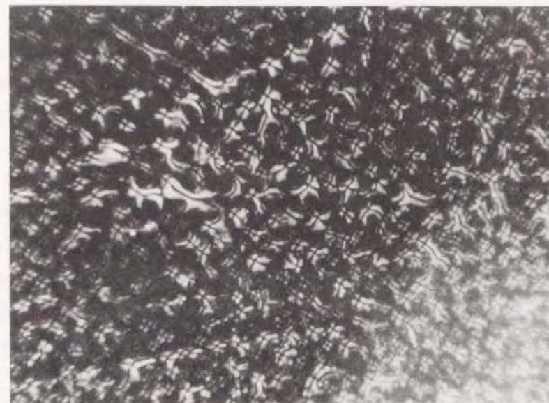
Figure 5. Smectic C schlieren textures shown by polymer B in the first cooling cycle at 96 °C, close to T_1 -s (Original magnification: 320 \times ).
