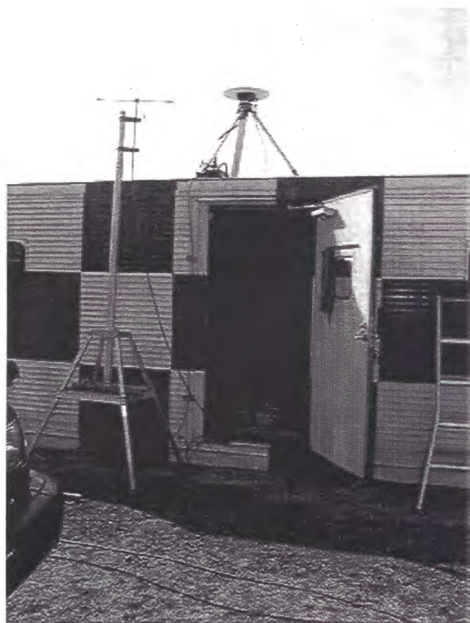
Fig.4-2 Ground monitor site, on which a Trimble Geodetic L1/L2 antenna was mounted, and the antenna of transmitter
