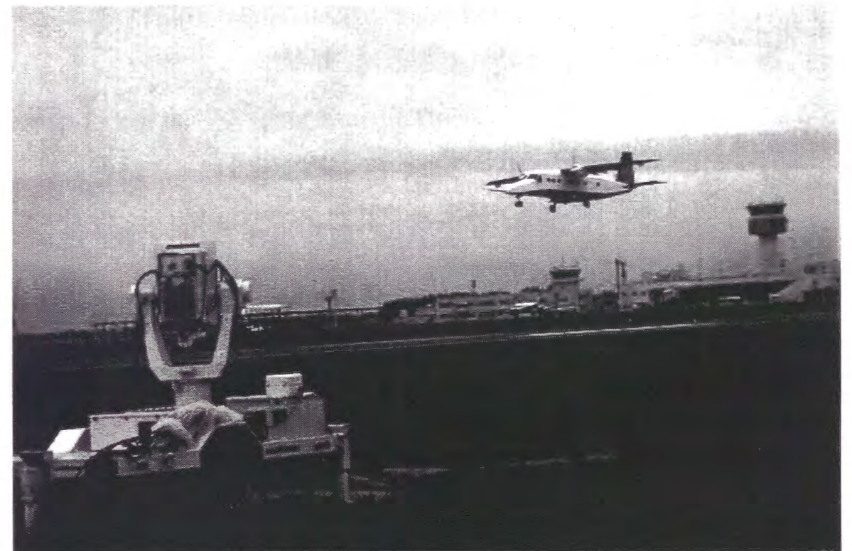
Fig.4-1 Research aircraft Do-228 and the laser tracker
