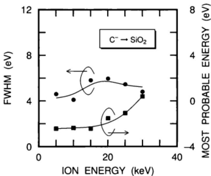
Figure 2.24 FWHM and most probable energy of the energy distribution as a function of ion energy in negative-carbon-ion impact on the  $SiO_2$  film of 120 nm thick at an ion current of almost  $2 \text{ nA}\cdot\text{cm}^{-2}$ .
