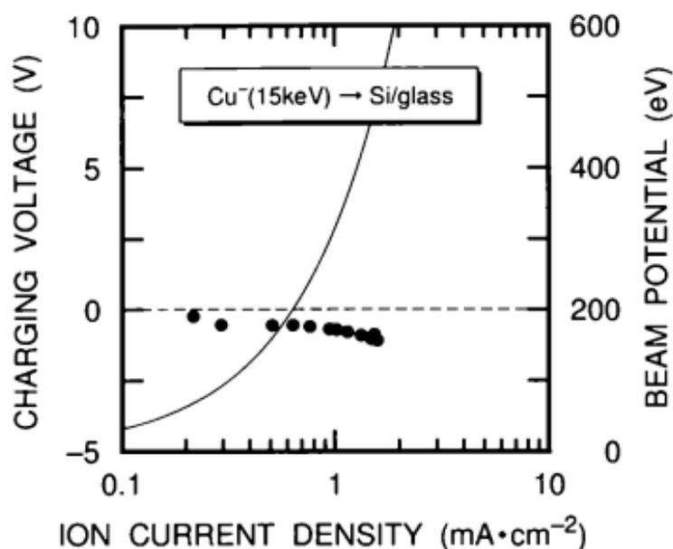
Figure 3.11 Charging voltage of the isolated electrode (Si/glass) as a function of ion current density around  $1 \text{ mA}\cdot\text{cm}^{-2}$  during negative-copper-ion implantation. The solid curve designates the magnitude of beam potential formed by an incident negative-copper-ion beam.
