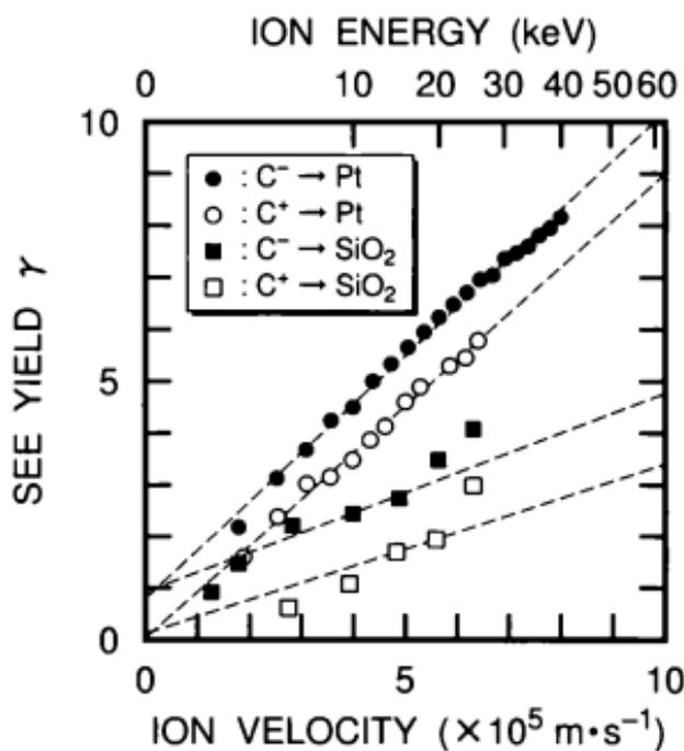
Figure 2.13 Yields of secondary electrons in positive- and negative-carbon-ion impact on platinum and  $\text{SiO}_2$  as a function of ion velocity. The broken lines designate the results obtained by the least squares method.
