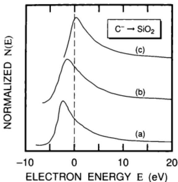
Figure 2.23 Normalized energy distributions of secondary electrons when negative carbon ions at ion energies of (a) 10 keV, (b) 20 keV, and (c) 30 keV with approximately  $2 \text{ nA}\cdot\text{cm}^{-2}$  were irradiated onto the  $\text{SiO}_2$  film of 120 nm thick. The horizontal axis is taken as the electron energy measured from the vacuum level at the retarding electrode.
