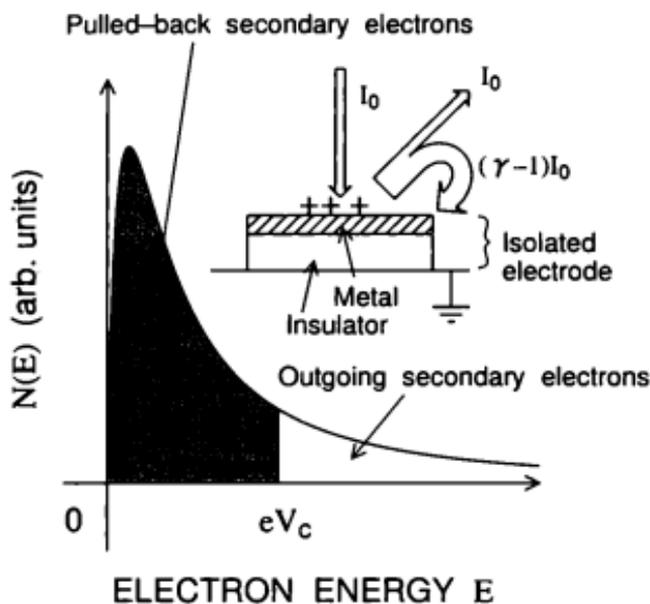
Figure 3.9 Schematic diagram illustrating the charge equilibrium of an isolated electrode during negative-ion implantation. In the charge equilibrium, the negative ions,  $I_0$ , are implanted into an isolated electrode; the secondary electrons with an energy of more than  $eV_c$ ,  $I_0$ , move away from it and the others with lower energy,  $(\gamma - 1)I_0$ , are pulled back to it.
