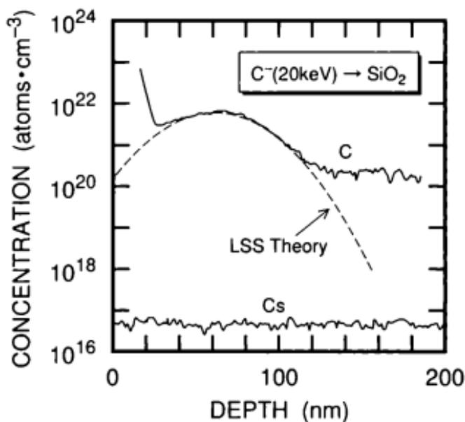
Figure 1.2 Depth profile of implanted carbon atoms in negative-carbon-ion implantation into a silicon dioxide substrate at an energy of 20 keV with a dose of  $1 \times 10^{16}$  ions·cm<sup>-2</sup> without any charge neutralization[35]. The cesium atom signal consists in the noise level.
