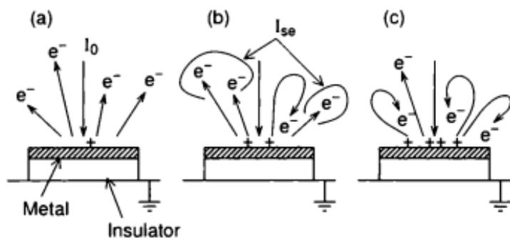
Figure 3.8 Secondary-electron trajectory and positive-charge accumulation on the electrode surface (a) at the beginning of ion implantation ( $|I_{se}/I_0| = \gamma > 1$ ), (b) after brief implantation ( $\gamma > |I_{se}/I_0| > 1$ ), and (c) in the charge equilibrium ( $|I_{se}/I_0| = 1$ ).
