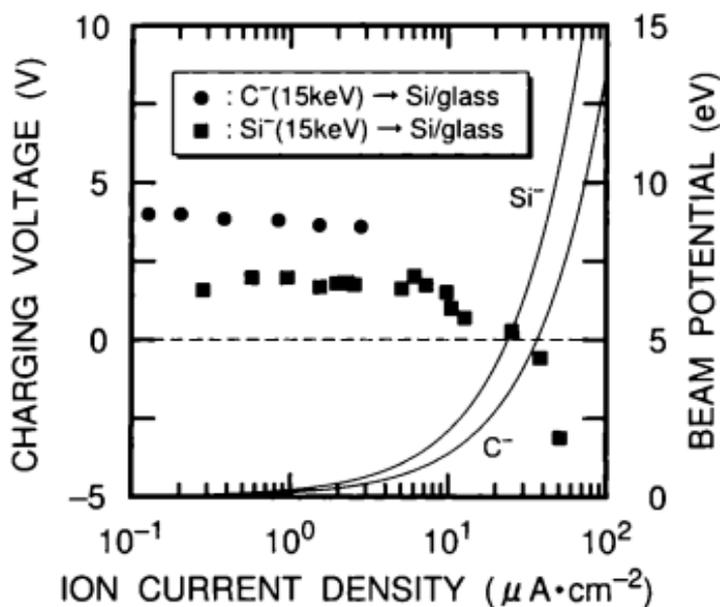
Figure 3.6 Charging voltage of isolated electrodes as a function of more than  $0.1 \mu A \cdot cm^{-2}$  ion current density in negative-carbon- and silicon-ion implantation. The solid curves denote the magnitude of beam potential formed by space charge of an incident negative-ion beam.
