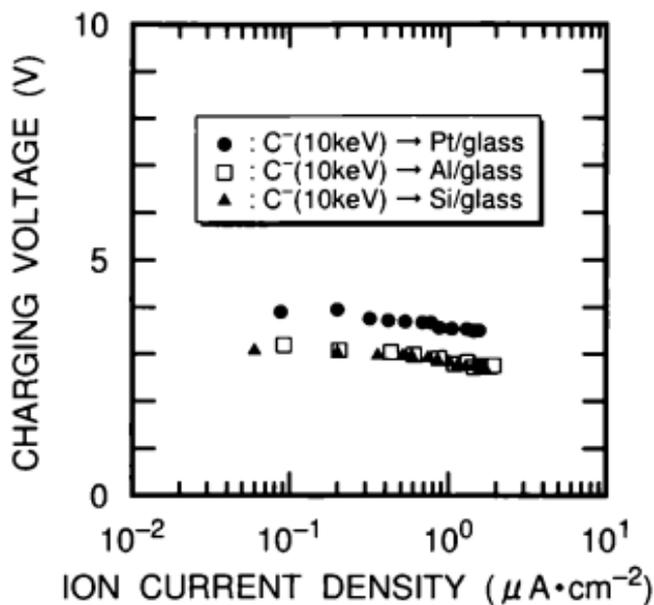
Figure 3.5 Charging voltage of isolated electrodes as a function of ion current density below  $1 \mu\text{A}\cdot\text{cm}^{-2}$ , in negative-carbon-ion implantation into Pt/glass, Al/glass, and Si/glass.
