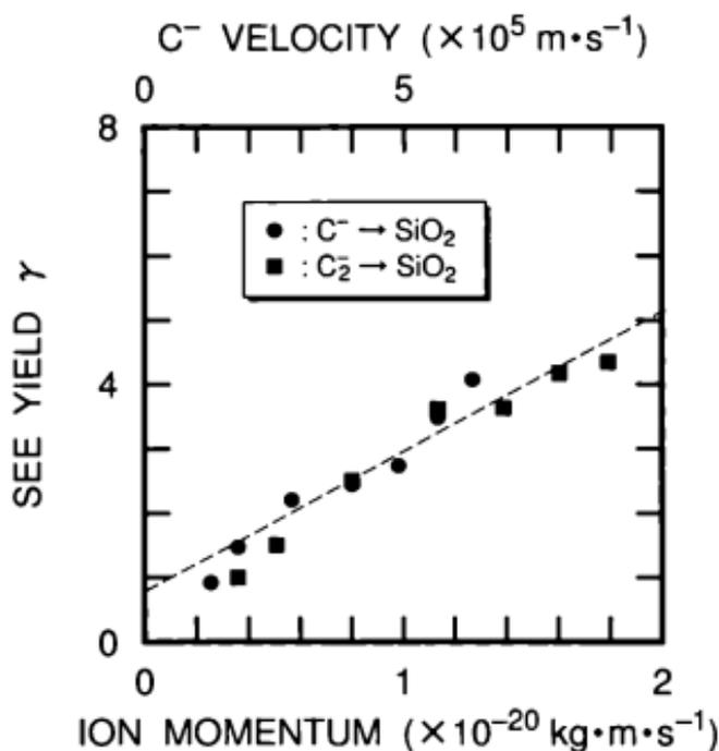
Figure 2.11 Yield of secondary electrons emitted from the  $SiO_2$  film as a function of ion momentum in negative-carbon-ion bombardment. The upper horizontal axis designates the ion velocity of monatomic carbon ions, which is twice the velocity of diatomic carbon ions. The broken line is obtained using the least squares method.
