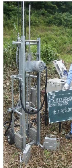
Figure 1. Hardware components of NSWS (Nippon Screw Weight System) testing machine
