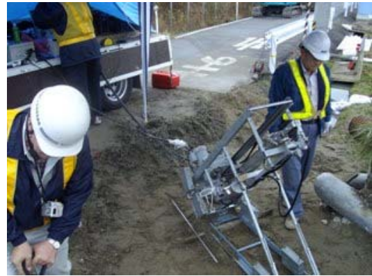
Figure 3. Appearance of inclination measurement with NSW S testing machine
