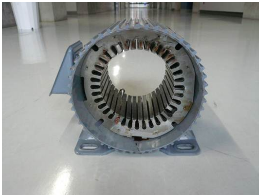
Figure 11 Photograph of stator core (slot number: 36)
