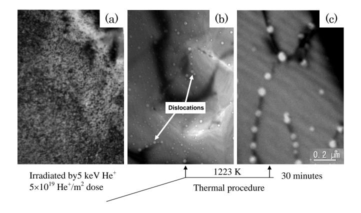
Fig.6. Microstructures in nickel after helium ion irradiation by 5.0 keV to  $5\times10^{19} \text{ He}^+/\text{m}^2$ : (a) heating to 1123 K at a rate of 1 K/s, (b) annealing at 1123 K for 1 hour, (c) re-heating to 1223 K, and (d) re-heating to 1263 K.
