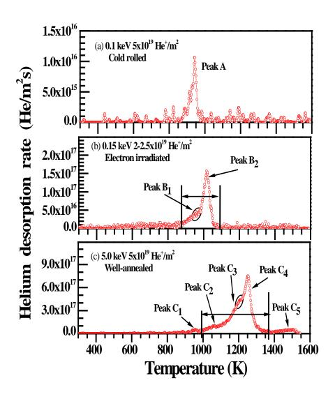
Fig.4. Helium thermal desorption and retention spectra in well-annealed nickel after helium irradiation by 5.0 keV to  $5 \times 10^{19} \text{ He}^+/\text{m}^2$ . Heating rate is 1 K/s, (a) was annealed at 1223 K for 1 hour, and (b) was annealed at 1123 K for 1 hour.
