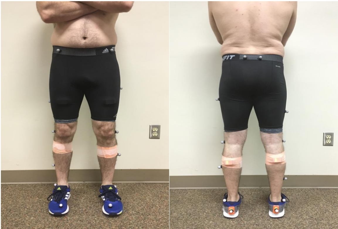
Figure 3.1. The placement of the IMU sensors and the retro reflective markers
