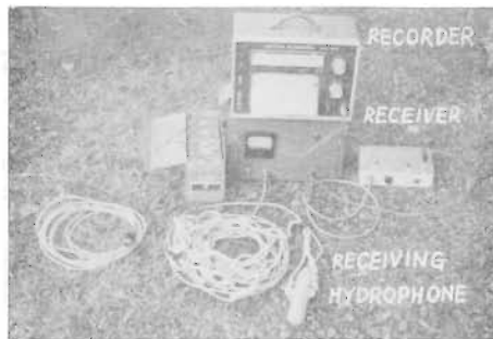
Fig. 4. General view of the deck unit (receiving hydrophone, demodulator and recorder).
