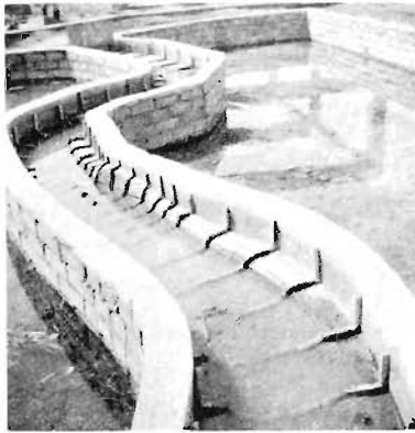
Photo. 2. Model channel with artificial roughness.
