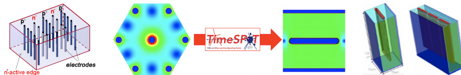
Figure 7.10: Geometry and weighting field comparison for 3D column and 3D trench sensor geometries [67].
