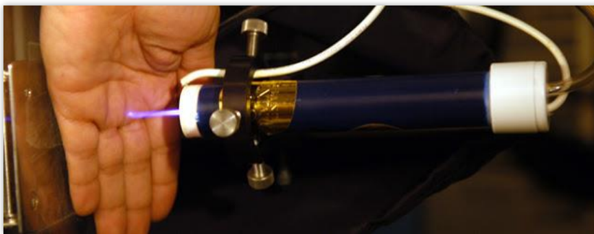
Fig. 3.11. Cold atmospheric plasma torches.
