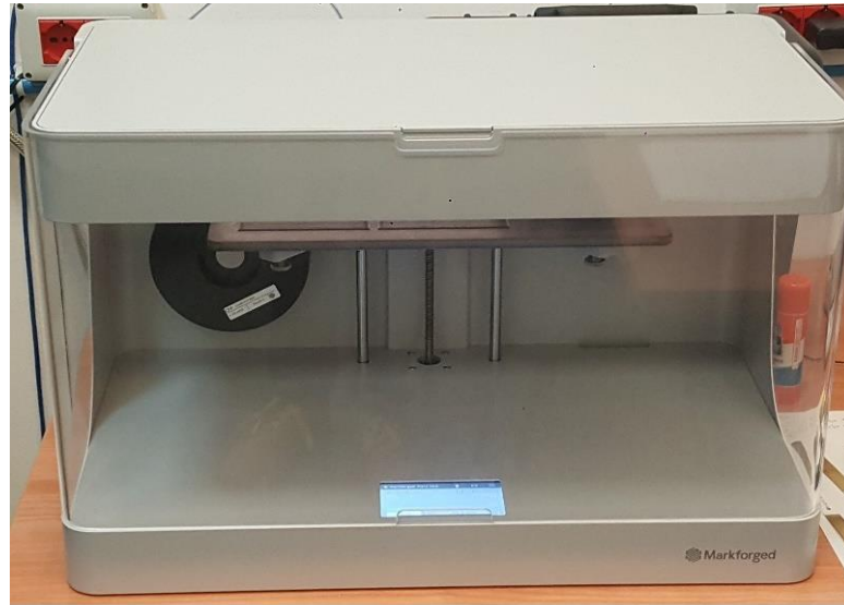
Fig. 4.27. The Markforged® Mark Two FDM desktop 3D-printer at the IIT laboratories.
