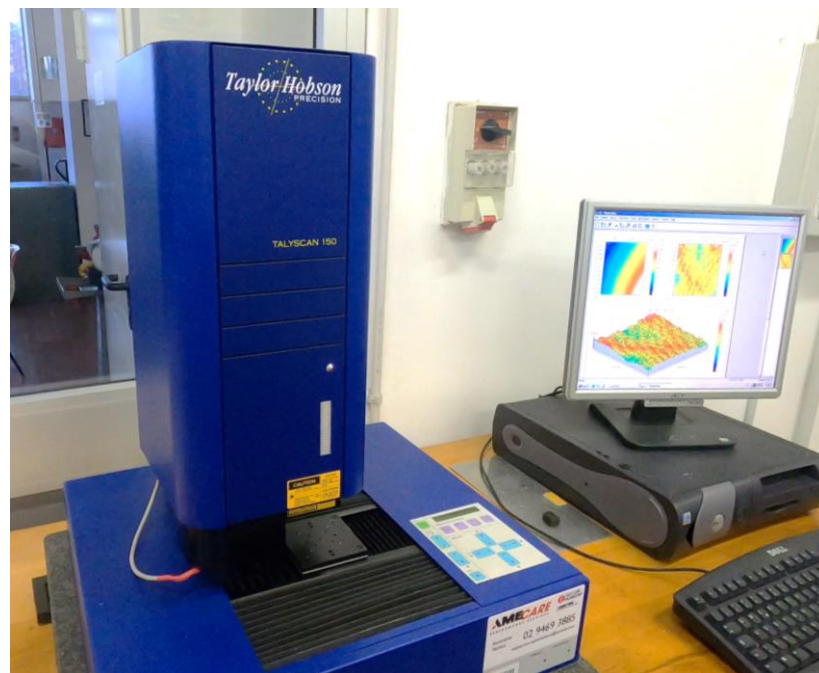
Fig. 4.40. Talyscan 150 laser profilometer.
