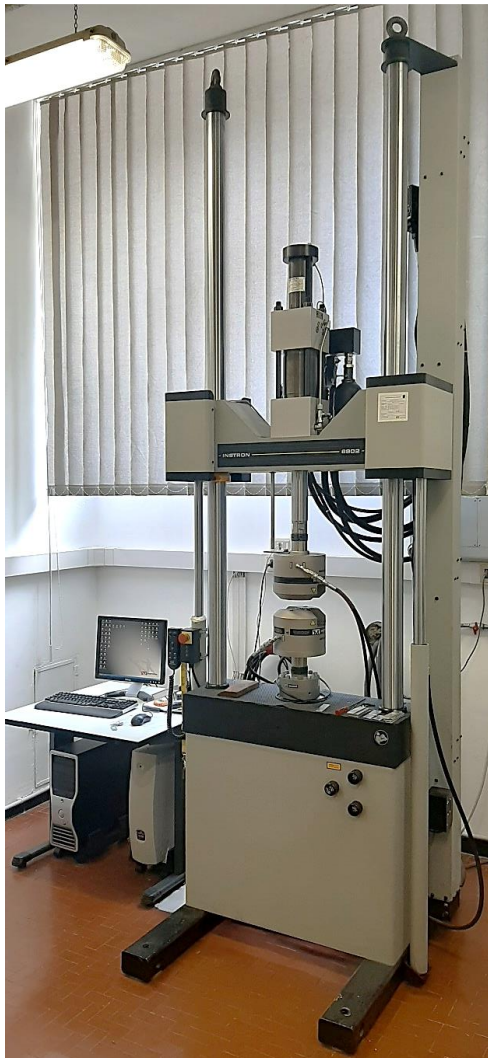
Fig. 4.15. Instron 8802 universal testing machine and detail of the gripping system.
