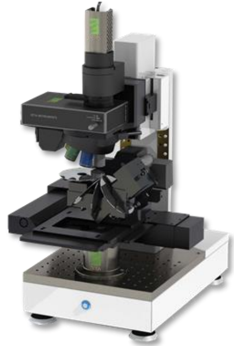
Fig. 4.17. Zeta20 3D optical profilometer.
