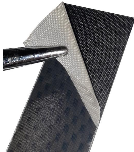
Fig. 4.5. Removal of the polyester ply from the peel-ply composite substrate.
