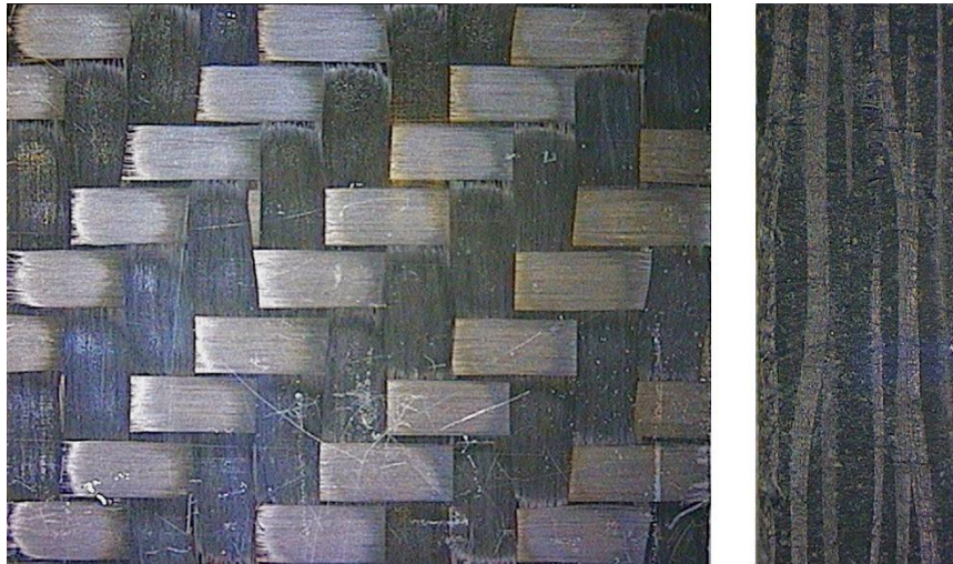
Fig. 4.2. Top view and cross-section of the CFRP used in Part B .
