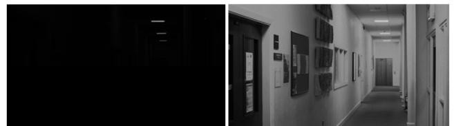
Fig. 11. Indoor natural test scene images captured for the proposed minimal images multi-exposure method for HDR image recovery. Exposure times: Left image: 888 \mu\text{s} and Right Image: 88.8 ms.
