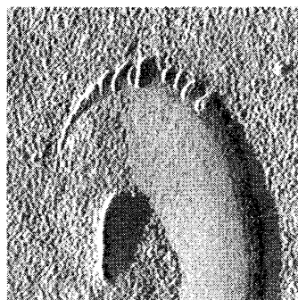
Fig. 2 AFM image of a polyethylene single crystal grown from the melt with tip splitting at a certain wavelength.
