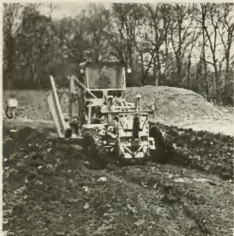
Fig. 2. Raw sludge is mixed with wood chips in the ratio of three parts wood chips to one part sludge.
