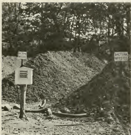
Fig. 6. A small cage fan draws air through the pile for 21 days. Temperatures of up to 82^{\circ}\text{C} . ( 180^{\circ}\text{F} .) have been measured in the piles.
