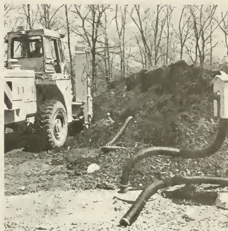
Fig. 7. After the 21 day composting period, the piles are broken down and new piles constructed.
