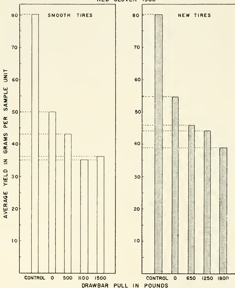
Figure 6. Effect of increasing drawbar pull with smooth tires and new tires on yields of red clover (1960).
