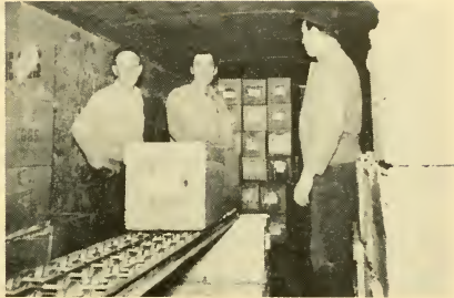
Figure 6. Time and effort may be saved in loading eggs in a trailer truck by the use of a loading device. The cases are placed on the roller in the warehouse (above), rolled into the truck (right), and then placed in position for shipment (below).
