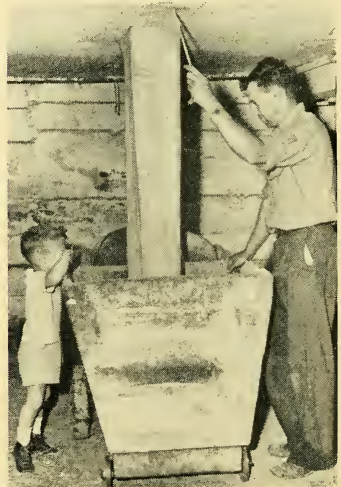
Fig. 17. The operator is pulling the rope that will fill the grain cart in half a minute or less. This is the same farm as diagrammed in Fig. 14.
