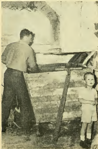
Fig. 45. This sawdust cart is filled quickly by gravity from an overhead bin.
