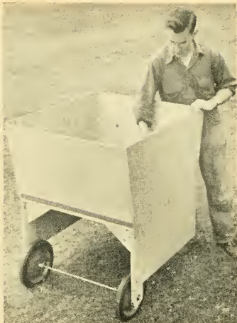
Fig. 18. One design for a grain cart. Note that the grain is at a convenient height for the operator. It is light and handles easily. It was built under the supervision of Paul A. Gilman, UNH Assistant Professor of Agricultural Engineering.
