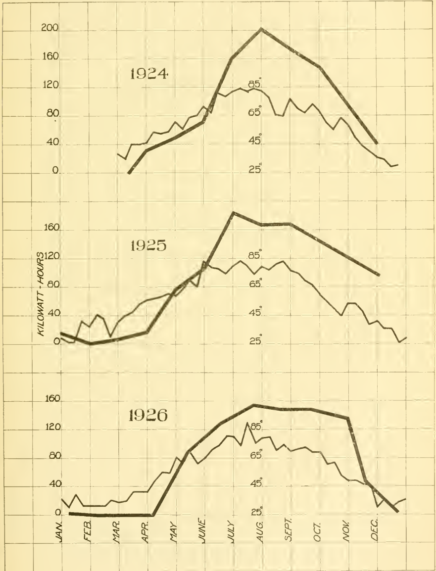
FIG. 3. Current consumption and outside temperature curves for 1924, 1925 and 1926 on Farm No. 2 showing the relation of the two factors. Kwhs. appear as the heavy curve and degrees fahrht., as the light curve.
