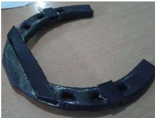
Figure 14. A prototype of optimal design of horseshoe (40% rubber pads)
