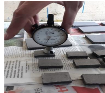
Figure 3. Specimen Surface Roughness Testing Process
